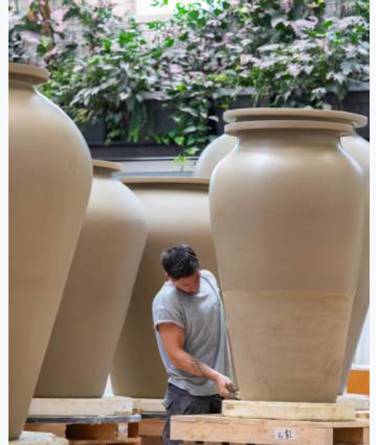
TAVA production site in Mori Trentino where vegetation is used to provide a more oxygen rich environment for their artisans and more consistent amphorae drying conditions.
