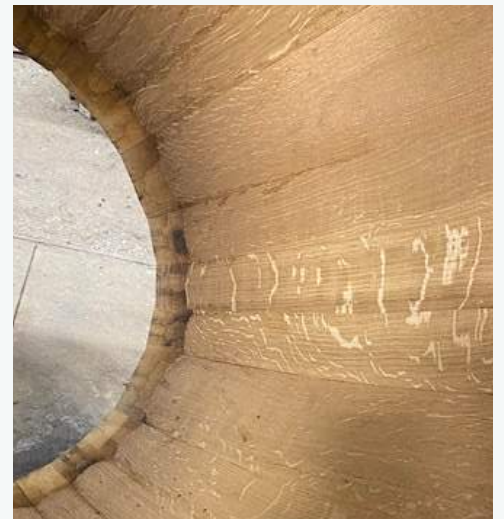
Noisette color of the inside of a DAMY barrel after the 2 hour super light long "Imperial" toast.
