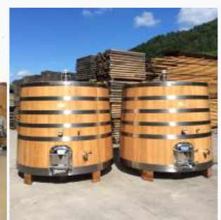
50 HL Conical operating tanks.
