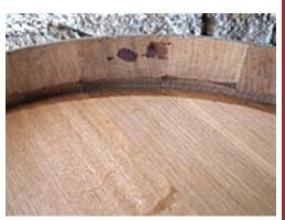
**2.** The first step is to use a hammer and a "scratch awl" (spile-shaped punch) to make a hole where you see the leak, to accommodate the spile.
