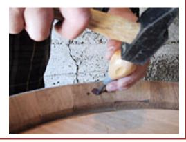
**3.** Next, you snip off the end of the spile if it is too pointy (need it blunt) and insert it into the hole. Use a hammer to tap the spile into the hole you have made. It should fit snuggly, but don't over do it.
